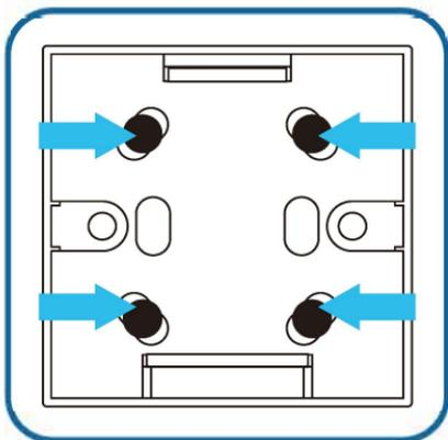
Securing the switch box to where you want to place with 4 Screws.
