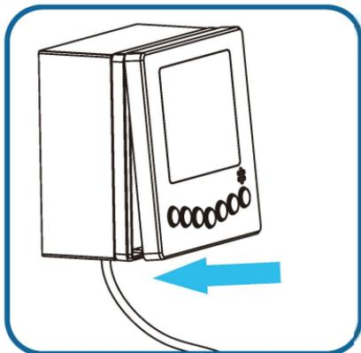
Install as the control board to switch box. Show below.
