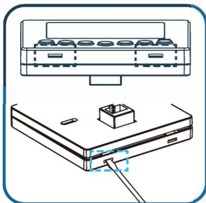
Softly poke these 2 slots with a flat blade screwdriver or the flat things, then open it by hand.
