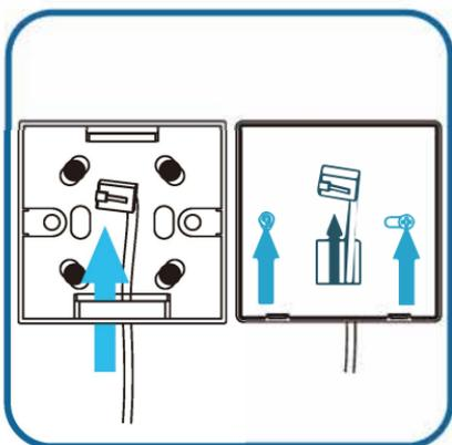
Putting the Wire through cover part and fix it on switch box with 2 screws.
